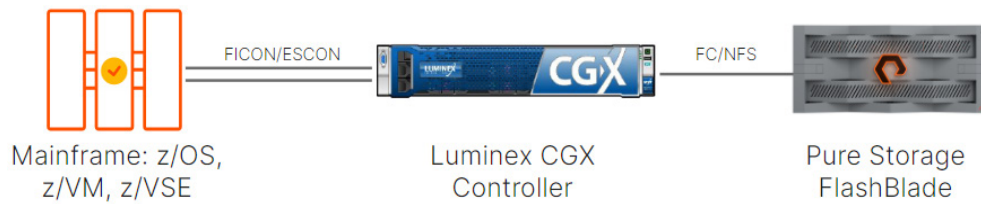
FIGURE 1 A basic virtual tape conceptual diagram. The mainframe is connected via FICON/ESCON to the Luminex GCX which emulates tape drives. The “virtual tape” data is stored on the Pure Storage device.
